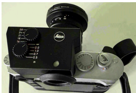
M11-P with 16-18-21mm lens and universal wide-angle viewfinder
