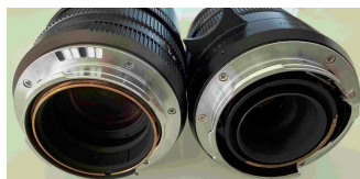
Figure 14: The white and black binary mark of the APO-SUMMICRON-M 1:2/75 ASPH lens on the left and the unmarked TRI-ELMAR-M 1:4/28-35-50 ASPH lens on the right.
