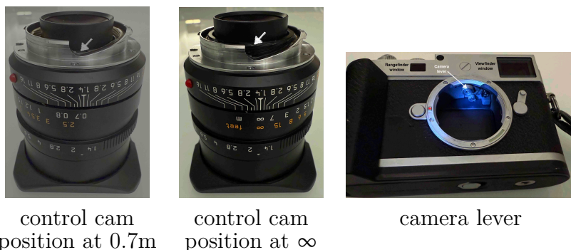
Figure 16: Mechanical link between the lens focus and camera
